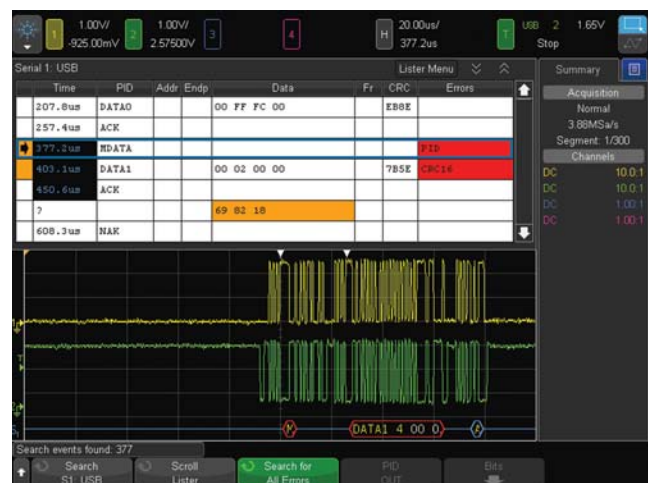
Figure 20: USB 2.0 trigger, decode and "lister" display.
