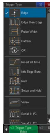
Figure 41: Wide array of advanced parametric trigger modes.
