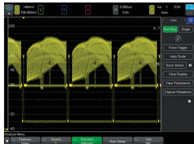
Figure 26: Triggering on 1080p HDTV signal analysis.
