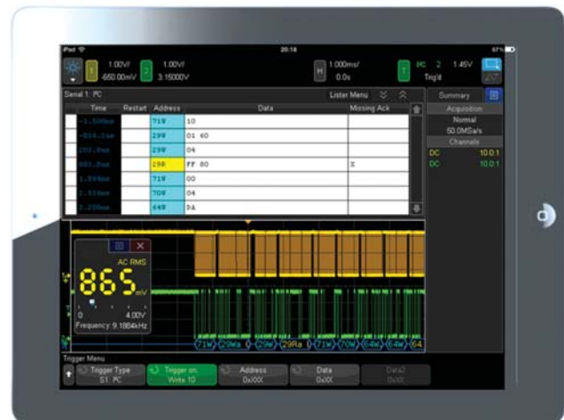
Figure 36: Tablet virtual front panel control.
