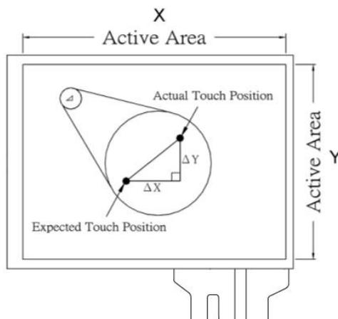
This test is to calculate the difference between the actual touch position and the expected touch position, which
