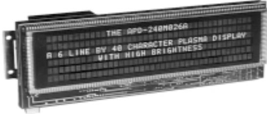
The APD-240M026A display module displays up to 240 alphanumeric 5 x 7 dot matrix characters arranged in 6 lines of 40 characters each. The module includes drive electronics and is easily interfaced to CRT controllers.
